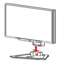
2. Connect the base into the neck of the monitor along the track.
