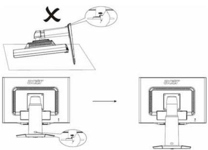
Slide the lock to right from the display support frame as per the figure and then adjust the height. Note that to slide the lock to right, erect the machine on the table to prevent the top part of the display from ejecting.
