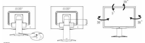
Do not perform a pulling or plugging action when the display is under slanting status to prevent the display from ejecting.
